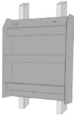
(A) Locate studs on 16" centers and attach with two wood screws provided
